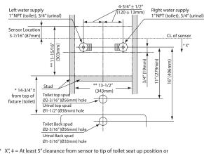
\* X", # = At least 5" clearance from sensor to tip of toilet seat up position of to top of grab bar is required to avoid false detection.
