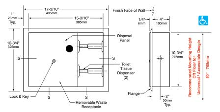
Rough Wall Opening 15-5/8" (395mm) wide 11-1/4" (285mm) high 4" (100mm) minimum recessed depth
