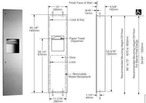
Rough Wall Opening 11-1/2" (290mm) wide 53-5/8" (1360mm) high 5-3/4" (145mm) minimum recessed depth
