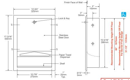
Rough Wall Opening 11-1/4" (285mm) wide 15-5/8" (395mm) high 4" (102mm) minimum recessed depth
